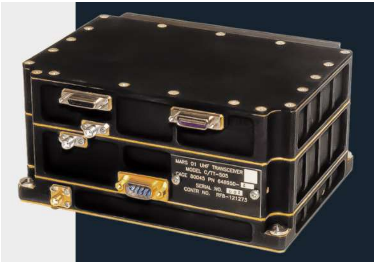
Electra Lite Mars UHF Transceiver - with familiar looking antenna sockets
